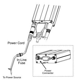
4. Connect the power supply cable into the power supply, with a correct GND connection.
